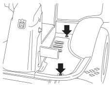
1 Loosen the locking nuts (1).
